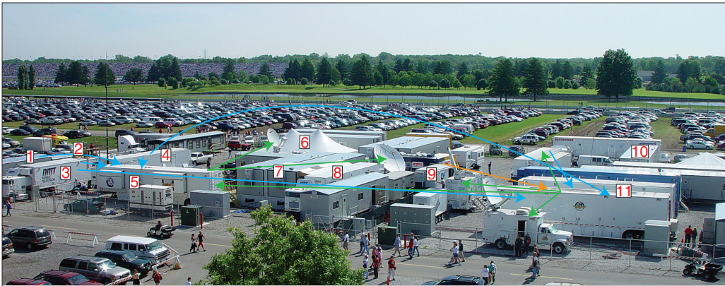
Figure 7.22 The infield television compound. An event this size commands an electronic village. The two trailers and Ku trucks on the near right side of the compound comprise the "international" feed, and provide the core coverage for everyone in the compound. This "international" coverage was provided by the track's own Indianapolis Motor Speedway (IMS) Productions (11). Behind the "international" camp are the trailers that comprised ESPN's coverage (10). ESPN covered the time trials, and put together prime-time programs right up to race day. The international camera contingent consisted of 33 cameras, not all of which could be housed in the IMS trailers, so some were the cameras that were on ESPN's NEP production trailer. RF cameras were provided by BST (1). In addition, there was one camera mounted on the Saturn blimp. The other half of the compound consisted of ABC equipment, anchored by NMT's DX-10 production trailer (5) and the DX-10T tape trailer (8). ABC also uses these two trailers for Monday Night Football. ABC took the international feed from IMS, and augmented it with almost a dozen additional cameras, namely RF handheld cameras roving the pits. Other trucks in the compound included a PVI virtual graphics truck (9), and BST's in-car camera control trailer (4), plus two additional Ku uplink (besides IMS's) and a C-band uplink truck. ESPN also had an editing and post-production truck from Location Solutions (blue trailer, right bottom area). Other compound support (2) and (3) – utility trailers; (6) – canteen tent; (7) ABC editing and tape library.
