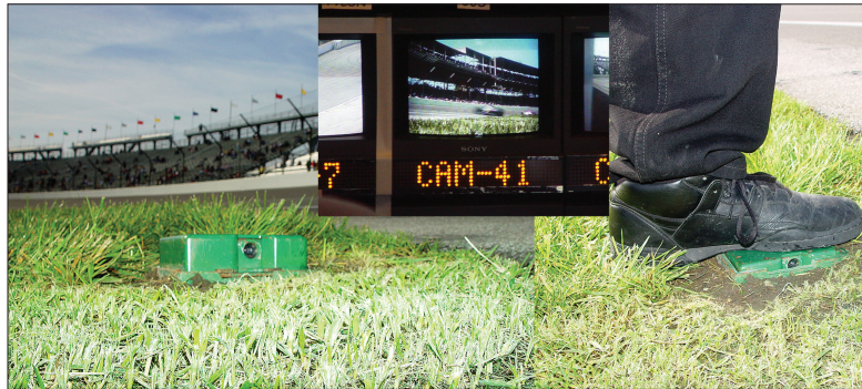
Figure 7.26 "Squash Cam" - Miniature POV camera just off the track that allows the viewer a sense of how fast the cars are moving past a point on the track. Since it is so close to the track there is a chance a wayward racer could run over it, so the camera is mounted on a spring assembly designed by IMS. It is sunk into the ground, allowing the camera to escape destruction if run over, or even just stepped on.
