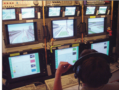
Figure 7.28 Inside PVI's virtual graphic truck. There was a dedicated PVI L-VIS connected to each of three cameras. One camera was used to provide inserts for the Start/Finish area. Another camera fed an L-VIS that did pit lane rendering, while the third camera fed a system providing virtual advertising on turn 4 of the track, which produced static images of a gooseneck sign that had ads for a couple of advertisers. Each of the systems is capable of inserting static, computer animations or live video with a live key. On the left monitor is an example of driver names being displayed alongside their pit locations. A flashing halo may be used in conjunction with this effect to highlight the pit stall area. The right side of photo shows the track/air temperature interactive graphic. All graphics use real-time tracking and may use occlusion processing (where not to apply the chroma keying) depending upon location and graphic use. PVI's system uses a combination of camera pan/tilt/zoom telemetry from the head, but they also have powerful video recognition software that can map the 3-D space that the camera is looking at into 2-D video space. The output of this truck is fed to the IMS production truck.
