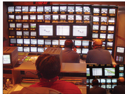
Figure 7.29 Monitor wall displaying 34 cameras and 34 VTRs available in the IMS production compartment, which is producing the international feed and the core racetrack coverage for ABC. The camera complement here includes eight cameras in cars and eight POV cameras. The director and producer will have their hands full during most of the race because under racing conditions the cars can travel the 2.5 mile track in under 40 seconds, and the story is told with approximately 12 camera cuts per lap. The inset photo shows the yellow flag tally above the program monitor, which gets its feed from the race control official. Race control is where the league officials monitor the race and control all aspects of the race. ABC has an associate producer in race control to determine the best time for commercial breaks based on what he observes and hears. Race officials use various feeds from the mobile units to make judgment calls.
